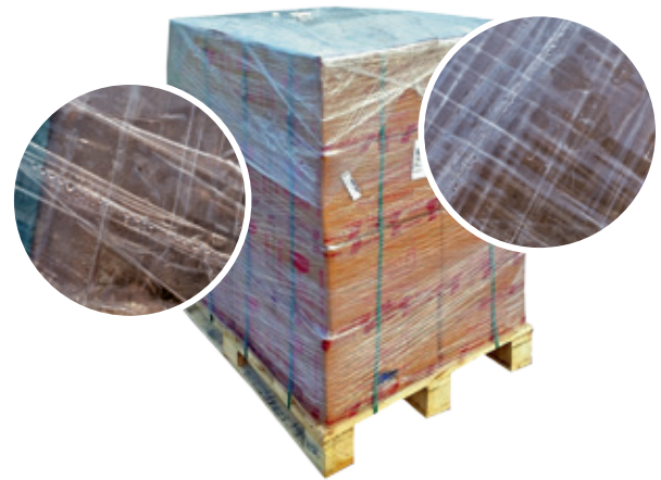
Condensation is clearly evident on a stretch-wrapped pallet following a seven-hour flight from Hyderabad to Oslo in moderate weather conditions.
